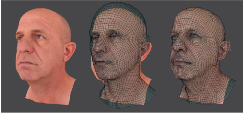
FIGURE 3 The template mesh warped to an input head model. A low-resolution template is shown for illustrative purposes
