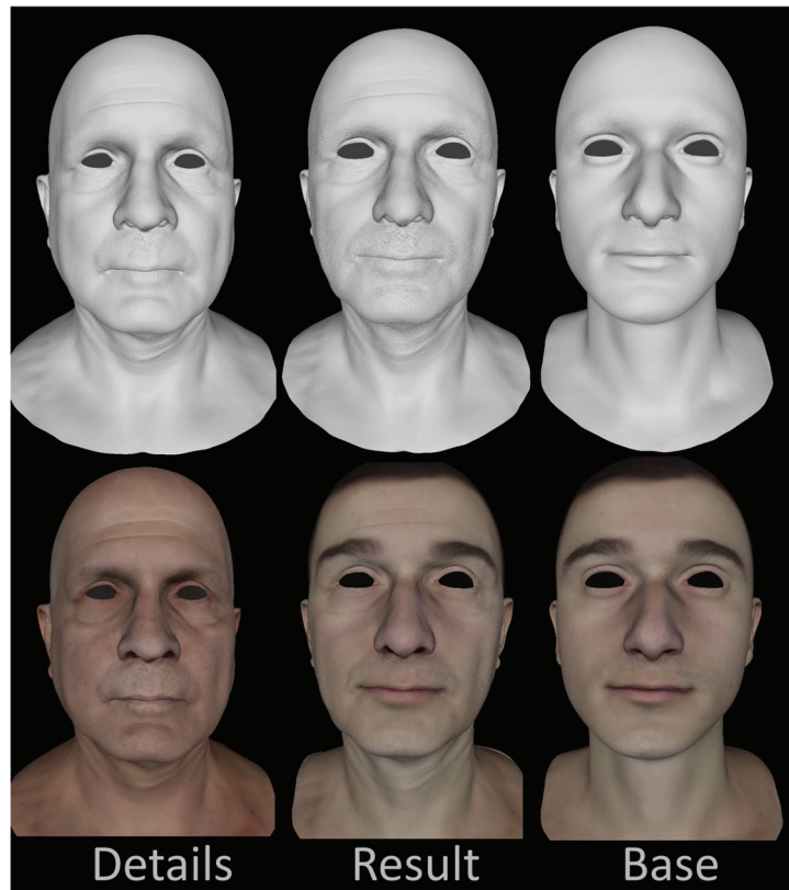
FIGURE 2 Result of blending two faces. The model on the left provides the details (source), the one on the right the base anatomy (target), and the result is shown in the middle. The textures are for illustration purposes only, our method only deals with geometric blending
