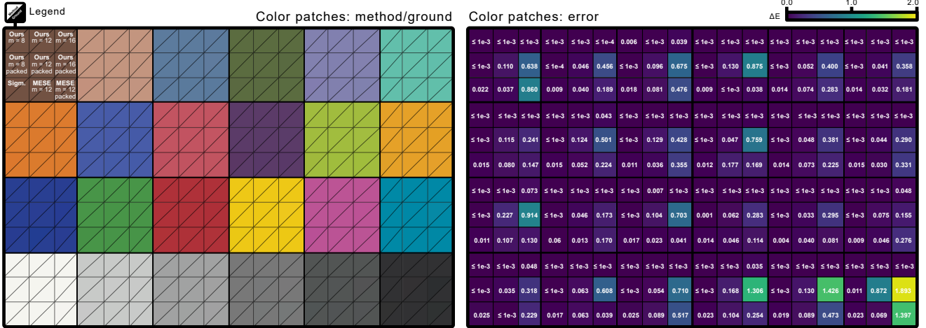
Fig. 10. Unconstrained color uplifting. We uplift color patches [BabelColor Company 2019] and render under D_{65} . Left . Output for our method ( m = 8, 12, 16 ), low-bit variants, the sigmoidal [Jakob and Hanika 2019] and the bounded MESE [Peters et al. 2019]. Right . \Delta E_{00} values are listed for all results.
