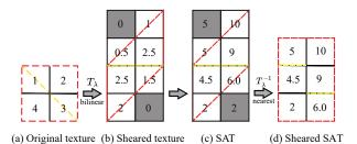
Figure 4: SSAT construction. (a) Original texture, (b) Vertical shear transformation with a bilinear sampler creates a sheared texture, (c) classical SAT, and (d) Inverse shear operation with a nearest sampler removes unused texels and produces our final SSAT texture.
