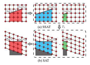
Figure 3: Our SSAT represents vertical integration under a line segment with a slope  $\lambda$  (a). We use shear transformation, to convert this problem to integration under a horizontal line segment which can be solved using SAT (b).
