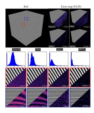
Figure 8: Checkerboard analysis. **Top:** FLIP error maps [2] show that both our method variants produce clearly lower errors than ANISO16, and EWAwhen compared to the ground truth reference (left top) in this texture minification task. **Middle:** Histograms of the full FLIP maps weighted by the error magnitudes as proposed by the FLIP authors [2]. **Bottom:** Two zoomed-in regions and their FLIP maps.
