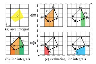
Figure 2: Integral over quadrilateral. We transform the area integral over a quadrilateral (a) into line integrals over its boundary (b). Then, we evaluate these 4 line integrals numerically (c). This method can be extended to arbitrary polygons.
