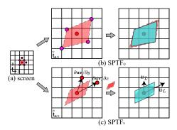
Figure 6: Pixel footprint approximation for SPTF. (a) A square screen-space pixel is projected to a quadrilateral Q in the texture space of the surface. (b) SPTF $_Q$ : A new quadrilateral  $Q_Q$  is constructed with edges following the nearest slopes  $\lambda'$  within our SSAT sampling space  $\gamma$ . (c) SPTF $_S$ : A semi-parallelogram  $Q_S$  is constructed by factorization of a covariance matrix.
