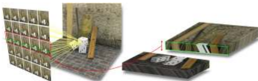
Figure 5.4: One way to visualize a 4D light field is to think of it as a collection of images of a scene, where the focal points of the cameras lie in a 2D plane. The rich structure becomes visible when one stacks all images along a line of viewpoints on top of each other and considers a cut through this stack (denoted by the green border). The 2D image one obtains in the plane of the cut is called an epipolar plane image (EPI) .
