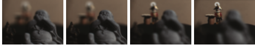
Figure 5.8: Example of a refocusing sequence. Left to right: the focal plane is moved from front to back, shifting the focus from the buddha statue to the pirate. The scene was captured with the kaleidoscope camera add-on [Manakov et al. 13] with an 50mm f/1.4 main lens. While this light-field camera add-on only captures nine directions, these views are sufficient to estimate depth and perform view interpolation, allowing for smooth out-of-focus blur.
