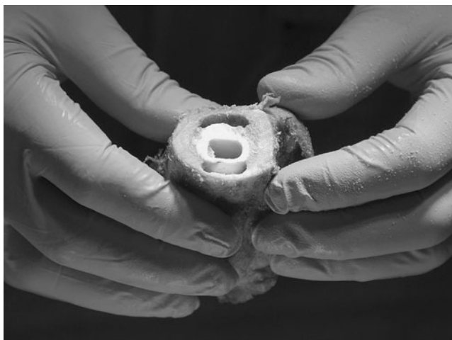
Fig. 4 Femoral lesions mechanically created anterior and posterior of the cement mantle are shown with the prosthesis removed
