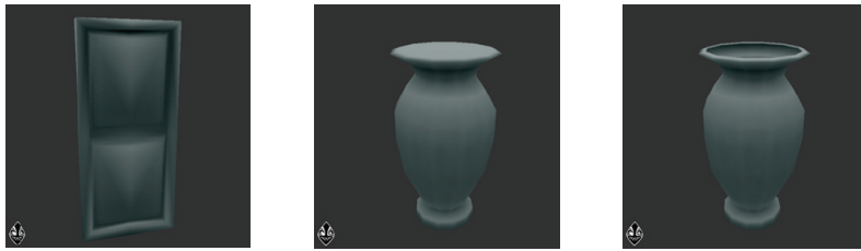
Figure 7 Base models for the examples in this section: a door (208 triangles), a solid vase (288 triangles) and a thin vase (576 triangles)
