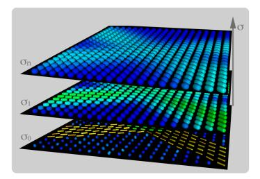
Fig. 2. Superquadric glyphs [20] illustrating Eq. (1) for five exponentially increasing scales  $\sigma_i$ . The synthetic DTI shows two fiber bundles crossing at a 65° angle.
