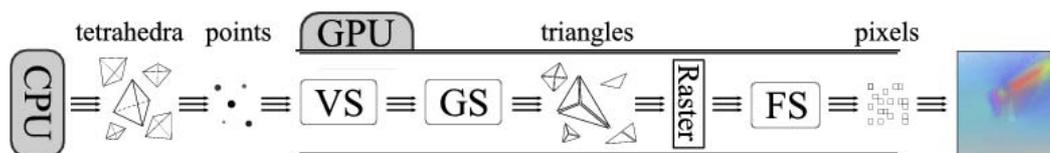
**Figure 4:** HAPT's pipeline: sorted tetrahedra are streamed as point primitives to the GPU; decomposed into triangles in the geometry shader (GS); and finally, during rasterization, the ray integral is computed per fragment to compose the final image.
