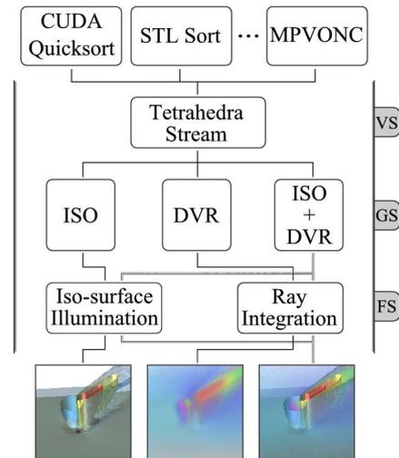
**Figure 3:** HAPT's Framework divided into vertex (VS), geometry (GS) and fragment (FS) shaders. Any sorting method can be used prior to rendering, for example: quicksort in CUDA; STL-based introsort on the CPU; or the MPVONC algorithm on the CPU (see Section 3.1 for details).
