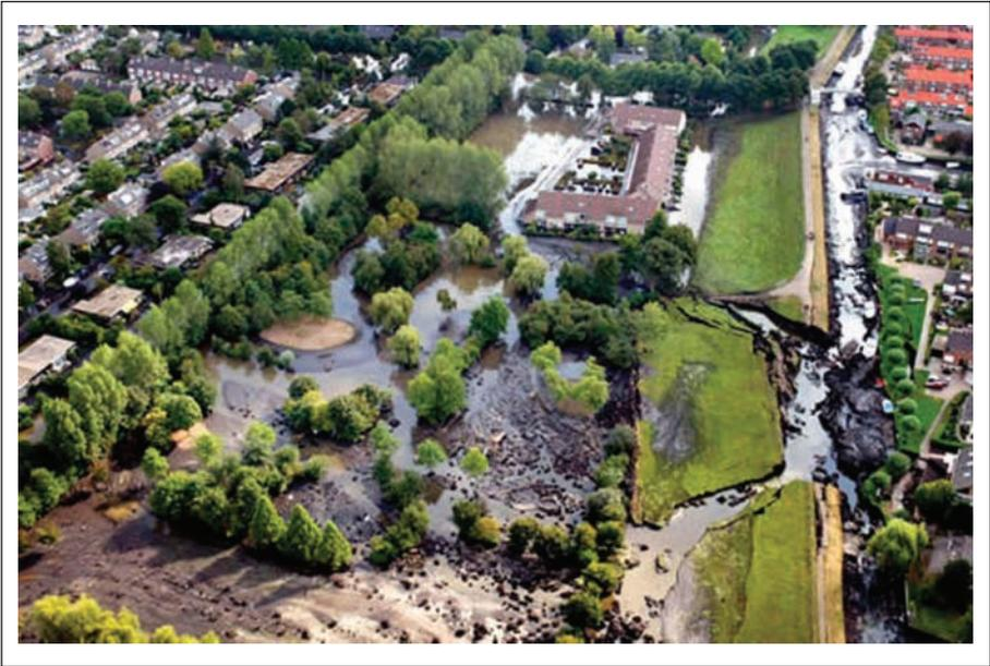
**Figure 1.** A Levee Failure in Wilnis, the Netherlands
