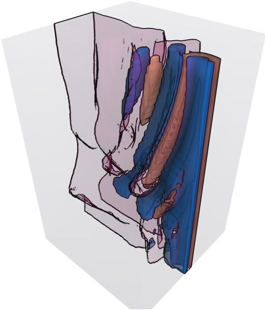
Figure 1: Illustrative visualization, created using our approach, of a multi-field representing the flow behind a tapered cylinder, placed vertically on the right side just outside the field. The field consists of the velocity vector field and its derivatives. The illustration highlights the alternating vortices characteristic for such flow. The transparent surface shows the area where flow velocity is altered by the cylinder.
