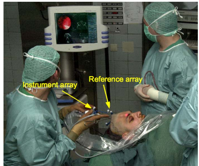
Fig. 10. Tracking of a surgical screw driver through an instrument array. Image is courtesy of Jürgen Hoffmann, Universität Tübingen.
