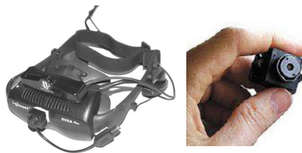
Fig. 1. HMD with tracker and micro-camera.
