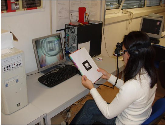
Fig. 6. The AR experiment with a clone copy of the image seen by the user on the monitor.
