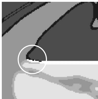
Figure 16: Typical classification result of the probabilistic method incorporating material mixtures of two materials.
