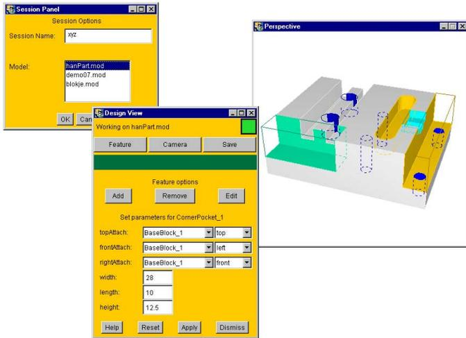
Figure 2 – User interface of a webSPIFF client: the user, working on a design view, is modifying some parameters of the corner pocket at the left side of the model
