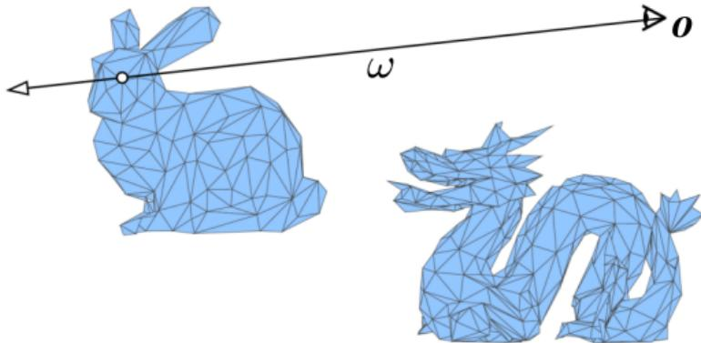
Use API to build acceleration structure for all scene triangles.
