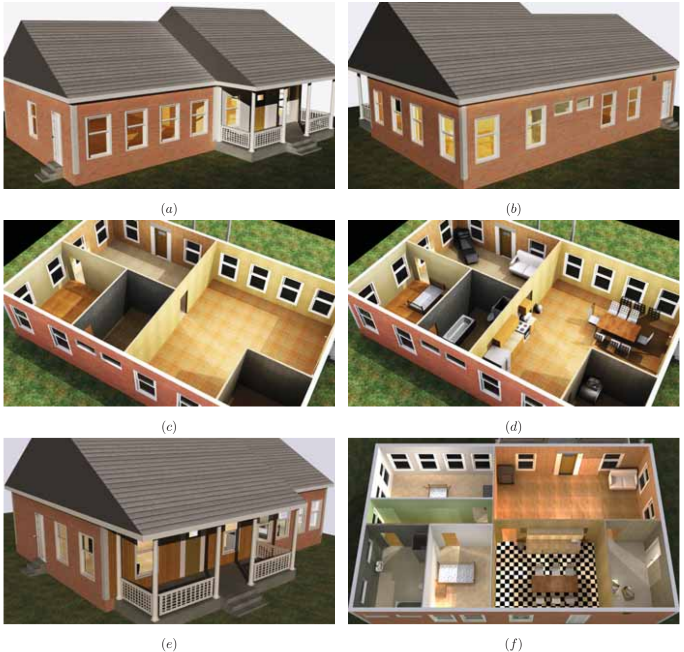
Fig. 3. Generation of a North American villa: (a) front view with porch; (b) back view with different types of windows and side-doors depending on adjacent rooms; (c) top view on the different rooms (great room, kitchen, bathroom, bed room, laundry); (d) automatically placed furniture based on room types and object relations; (e)-(f) front view and interior view of the same plan, but now using another floor plan generation technique, that of Marson and Musse [28].
