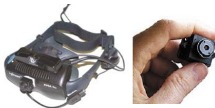
Fig. 1. HMD with tracker and micro-camera.
