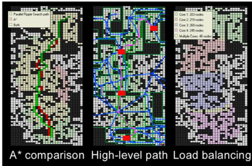
**Figure 12.** Path generated with the Parallel Ripple Search algorithm. (Left) Comparison with the classic A\*. (Middle) The high-level path used and the way-points used to start off the non-essential cores. (Right) Each core has flooded roughly the same amount of nodes. The yellow nodes indicated collisions.
