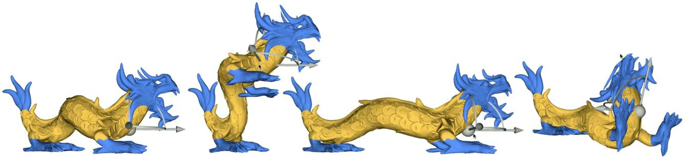
**Figure 2:** Interactive deformation-based editing of a Chinese dragon model with 260k triangles (see Table 1).
