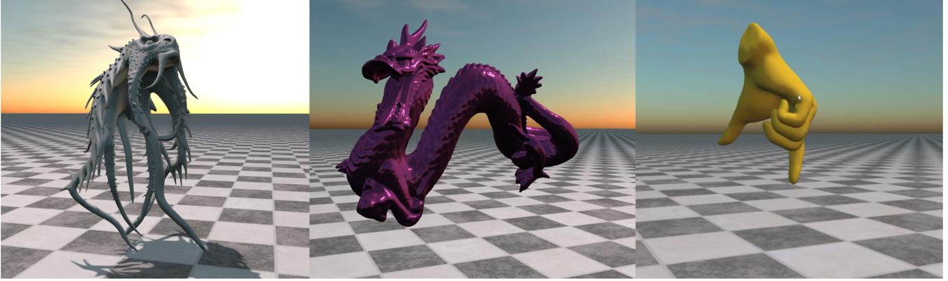
Fig. 2. Compilation of frames from three of the simulations shown in the **supplementary video**. The squid simulation (440k vertices, 1.6 million tetrahedrons) runs at 37 fps (including rendering and ground collision handling), the rest of the examples run at least at 60 fps.
