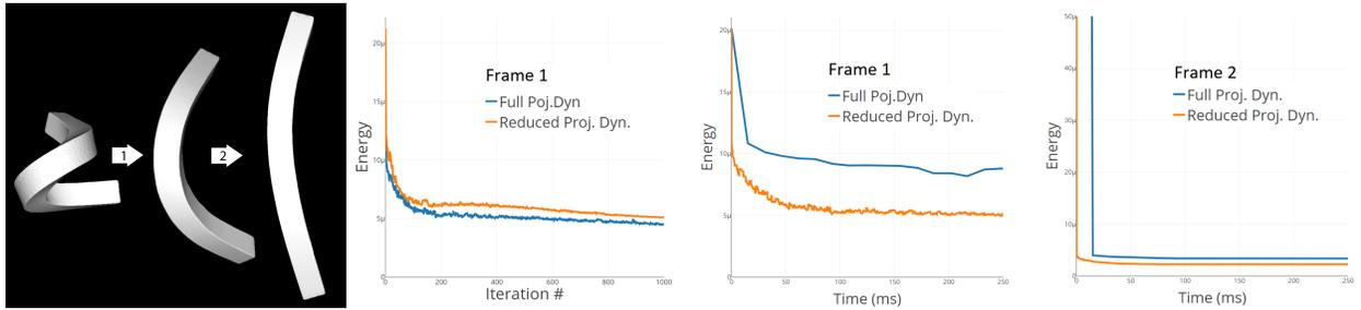
Fig. 3. Progress plots displaying the evolution of the objective (2) during minimization using the local/global solver for the full and the reduced problem. Large time steps are taken and the resulting frames are shown on the left. For the first time step, the objective value versus iterations *and* time are shown. For the second timestep, objective value versus time are shown.
