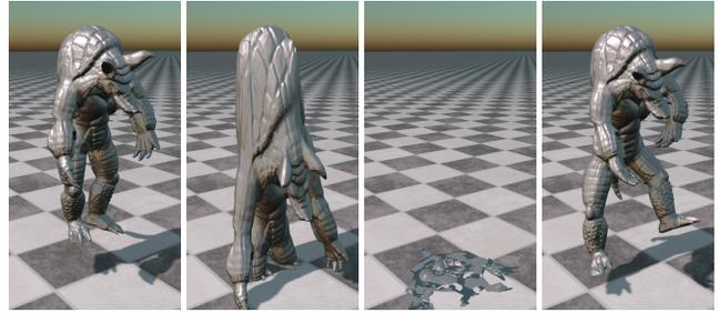
Fig. 6. We are able to interactively change stiffness parameters in a running simulation. From left to right we scale the predefined weights by 1, 0.1, 0 and again 1. This also demonstrates that our method is able to recover from a fully flattened state.
