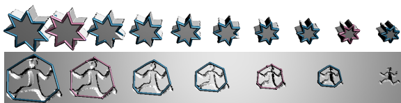
Figure 10: Although our descriptors are not scale invariant to increase precision, our method is scale tolerant (green) when learned (red) and supports complex features (top: discontinuities, bottom: embossed shapes).
