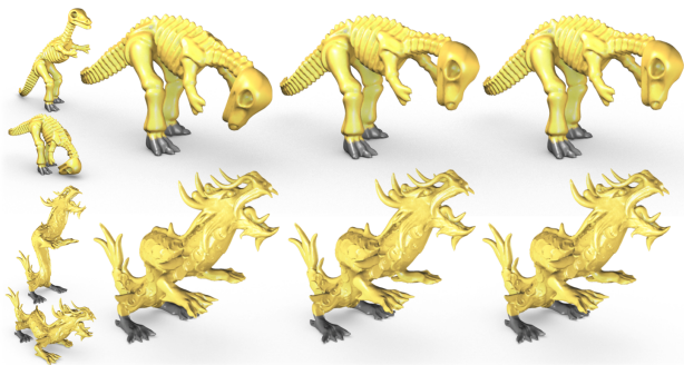
Fig. 7. Subspace fidelity. Mean shapes of the dinosaur and Chinese dragon model computed in spaces of varying size. From left to right: the two example poses, mean shapes obtained in a 3 dim., 17 dim., and unreduced space. (See Tbl. III for Hausdorff distances.)
