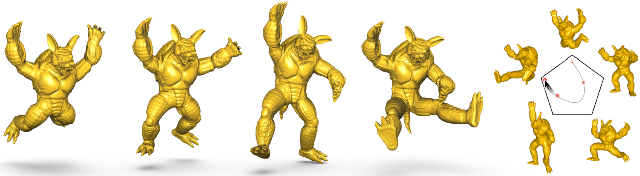
Fig. 1. Snapshots from an interactive shape interpolation session with five example poses of an armadillo shell model with 332k triangles. After a preprocess, our framework for nonlinear shape interpolation computes weighted average poses in real-time (see Table I).
