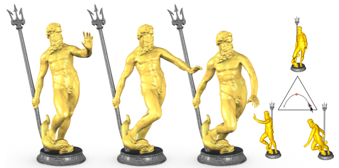
Fig. 2. Weighted elastic averages of three Neptune solids with 691k tets using the nonlinear Mooney–Rivlin material computed at rates around 100 interpolated shapes per second (see Table I).
