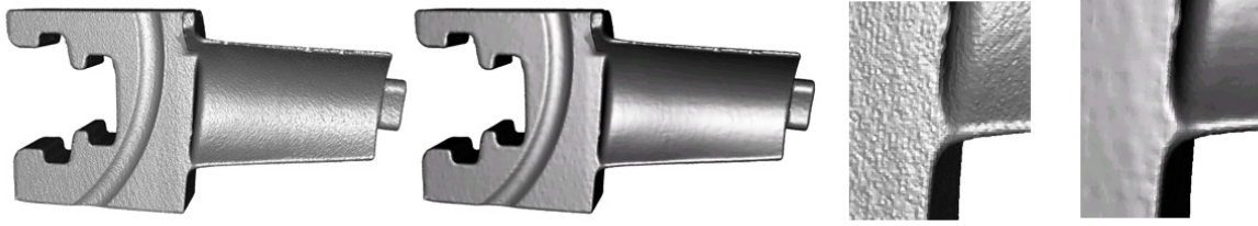
Figure 4: Noise removal from the scanned blade model with 390 k triangles. Details are shown on the right.
