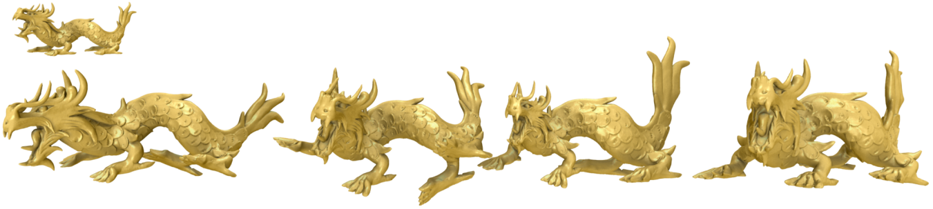
Fig. 1. Linear vibration modes and modal derivatives of the discrete shells energy on the dragon model. Figure shows: the rest state (top left), two linear modes (left), and two modal derivatives (right).
