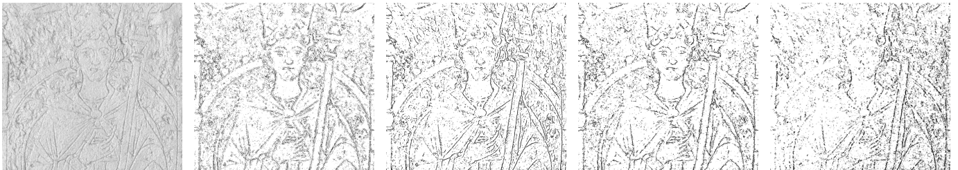
Fig. 15. Different feature line methods are applied to the model. From left to right: shading, ridges and valleys, suggestive contours, apparent ridges, and photic extremum lines.
